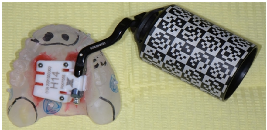
Patient tracker attached onto the denture duplicate
